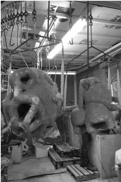
Ceramic investment molds at Bollinger Atelier. The sections of the statue are encased in heat-resistant ceramic in preparation for bronze pouring. The cylindrical tubes are the channels for the liquid bronze to pour through.
